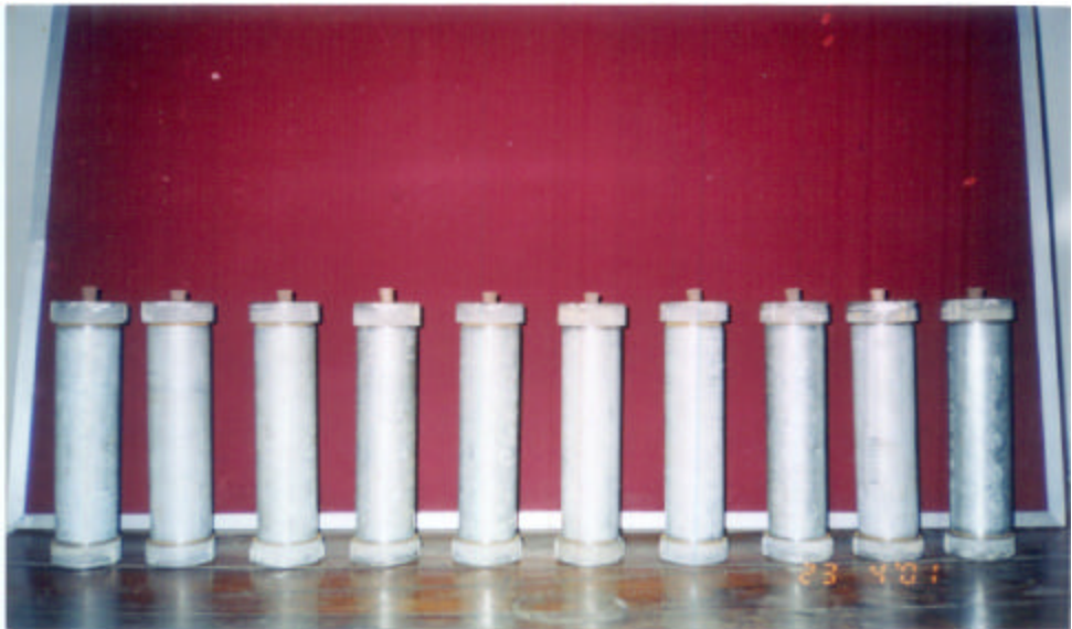
Figure 7: Setup of anaerobic digestion chamber for the arsenic wastes developed at BUET
