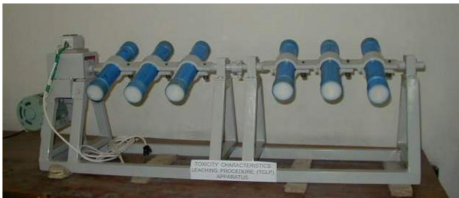
Figure 1: TCLP Agitation apparatus constructed at BUET
