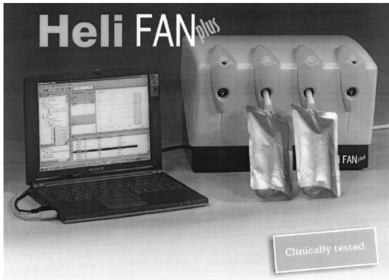
FIG. 1. FAN nondispersive infrared spectrometric ^{13}\text{C} -Breath test analyser HeliFANplus
