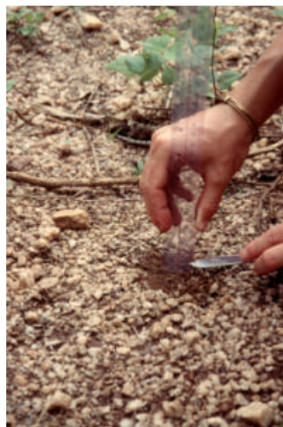
Figure 4.4b: Measuring Armour Layer Using a Ruler, Sri Lanka
